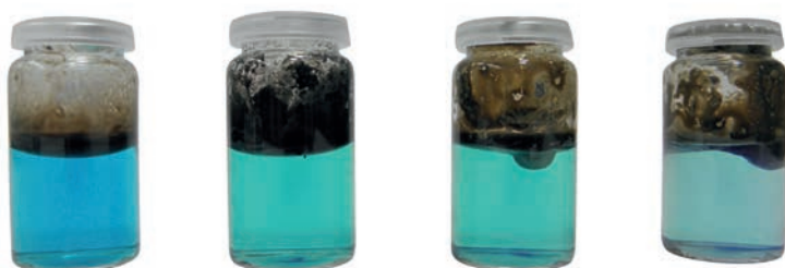
Examples of Different Total Iron Concentration Measured in cylinder drain oil (CDO) Samples
